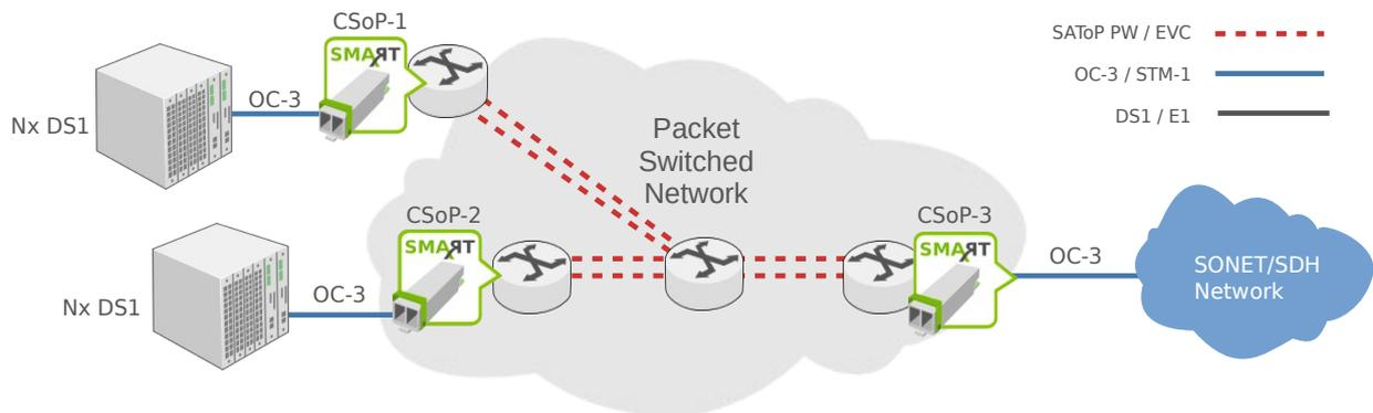
**Figure 5: Aggregate low-fill OC-3 from network edge**
