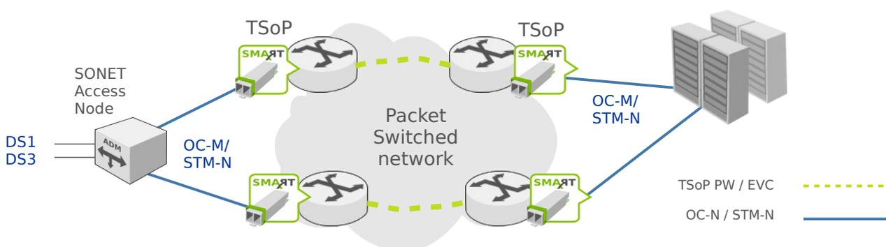
**Figure 6: SONET access via Clear-channel TSoP SFP**
