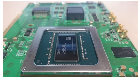
AimValley Designed 400G card with AMD Versal FPGA
